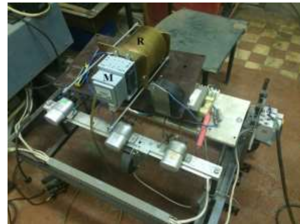
Fig.8. Experimental setup microwave plasma torch in air
