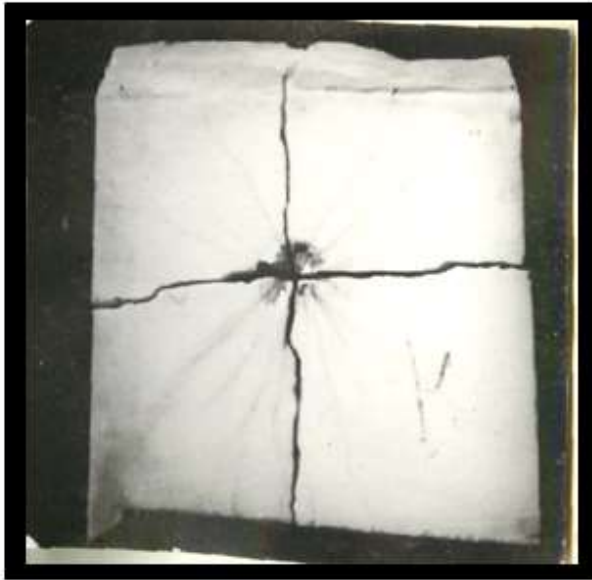
Fig. 8. The nature of destruction during electrical breakdown of cement samples
