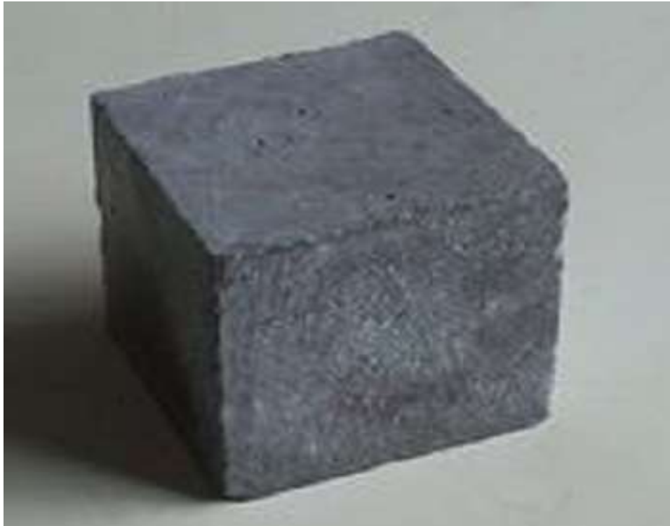
Fig. 7. Individual square concrete samples in the experiment.
