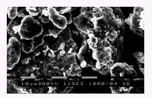
The powder mixture after 2 min MA. Particles adhered and grouped to each other. Such groups of deformed particles formed agglomerates.
