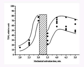
Figure shows the content of the TiNi phase in the product synthesized in the thermal explosion mode at different preliminary MA times.
