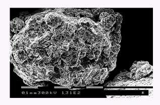
The powder mixtures after 4 min MA. The general trends in the development of agglomerates can be traced. Consolidation and compaction of agglomerates occurs with an increase in the MA time.
